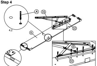
Fix the left & right hydraulic spacer together with hydraulic base supporter to the both side rails using bolts  ${\bf G}$  and than screw the minifix part  ${\bf A}$  to the both side rails as shown in diagram 4.2.
