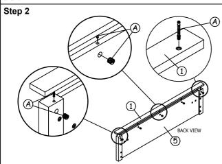
Firstly screw the minifit part A to the top bar (1) as shown and than fix the top bar (1) to the footboard frame (5) using hardware parts A.
