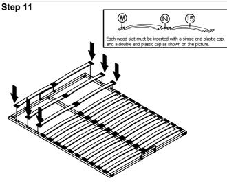
Insert the slats (15) to hardware parts  $\boldsymbol{M}$  and  $\boldsymbol{N}$  then press into the base making sure they are secure.
