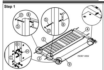
Attach the headboard frame (2) and back storage panel (9) to the left wooden post (3) and right wooden post (4). Secure the headboard frame using hardware parts **B**, **D** and **O**, then secure the back storage panel with hardware parts **B**,**H** and **I**.
