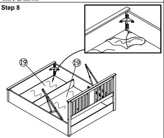
Attach Non-Woven Fabric Small and Big (19) at the bottom as shown in diagram.
