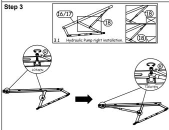
Firstly, Loosen the **Hex Nut** from the Left & Right Hydraulic Base Support , then fix the hydraulic pump to each hydraulic base using the same Hex Nut & V. (shown in diagram 3.1. )
