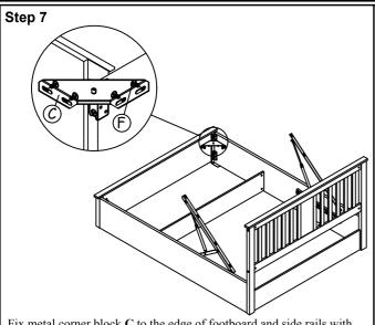
Fix metal corner block  ${\bf C}$  to the edge of footboard and side rails with bolt  ${\bf F}$  as shown.
