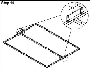
Attach hardware parts **J** using hardware part **K**. **Important note: Please assemble follow arrow direction.**DO NOT use any power tools as this may damage the frame and will invalidate any claim.
