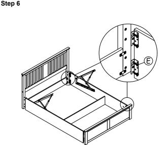
Fix side rail to the headboard and footboard with hardware as shown.
