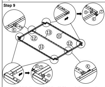
Join together all the bed base parts (11),(12), and (13) by using hardware parts **K,S,T**. **Important note: Please assemble follow arrow direction.**
