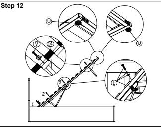
Assemble the bed base on the right & left hydraulic frame and fix bolts L starting from '1' to '3' as shown and fix the support leg (14) to the bed base as shown and than stick it the self adhesive U as shown. Important note: Do not tighten the bolts yet!
