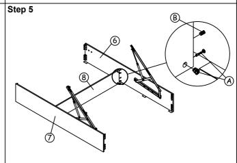
Join together the left side rail (6) and right side rail (7) with the centre storage panels (8) using hardware parts A and B.
